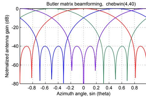
Fig. 4. Four spatial orthogonal patterns weighted with Chebyshev window.
