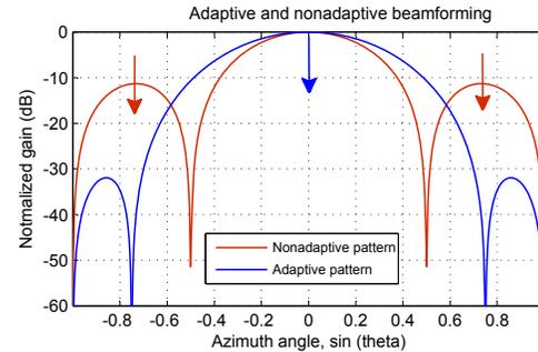
Fig. 5. Patterns formed by dominant eigenvector. Directions of arrival of desired and interferer signals are  $\theta_d = 0$ , and  $\theta_k = \pm 0.7$ , respectively.
