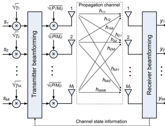
Fig. 1. Transmitter-receiver node pair in MIMO ad hoc network.
