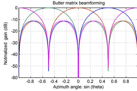
Fig. 3. Four spatial orthogonal patterns formed by Butler matrix.
